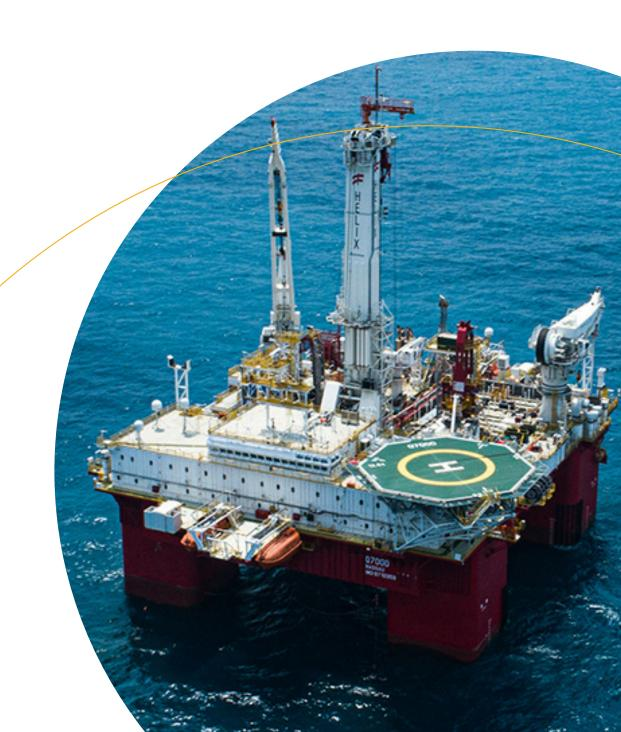
The Helix Q7000, a purpose-built DP3 semisubmersible vessel built to perform in harsh environments such as the North Sea, enables riser-based subsea well intervention and decommissioning operations.
